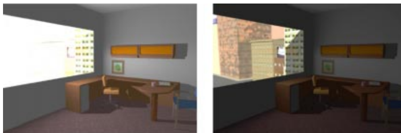
Fig. 3 An example of an HDR image displayed, keeping the details in interior (left) or exterior (right) levels of luminance readable.
