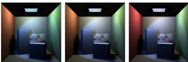
Fig. 13 Von Kries color correction for the A/C illuminants: CIE RGB (left), Stiles and Burch (center), and Thornton (right) CMFs.
