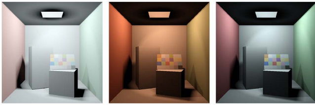
Fig. 9 Logarithmic mapping for the D65 illuminant: CIE RGB (left), Stiles and Burch (center), and Thornton (right) CMFs.
